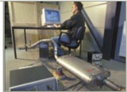
MIMO testing allows single or dual shaker and impact hammer FRF measurements.
