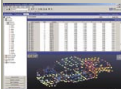
The geometry workbook allows fast generation of wireframe and full 3D visualization of test and analysis results of large models.
