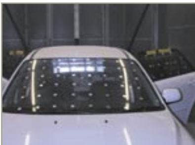
High channel count operational modal analysis allows detailed testing of large structures under operational loads.
