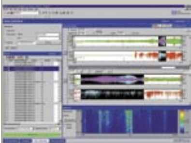
The display offers a convenient overview on all time histories and allows easy data selection for multi reference cross power processing.
