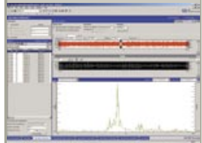
Starting from user-selected segments of time data, the time histories are processed into cross powers for parameter estimation.
